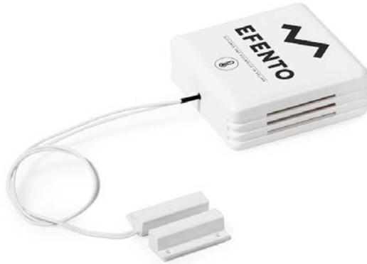
Wireless open / close sensor monitor, log in their memory and transmit over Bluetooth Low Energy events of door opening and closing. The sensor is equipped with a magnetic sensor which can be plastic or metal.
